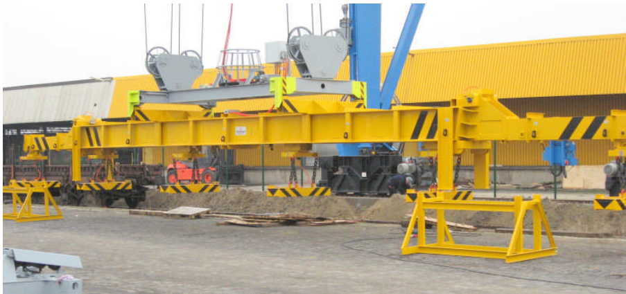
Figure 2: Fixed spreader beam for carrying thick plates with travelling magnets and removable extension arms; spreader beam is coupled to a container lifting device
