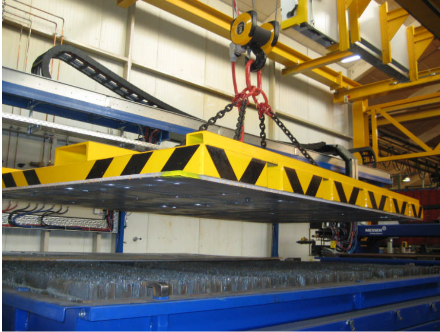
Figure 3: “Magnetic carpet” for loading and unloading large-format plates in a single lift
