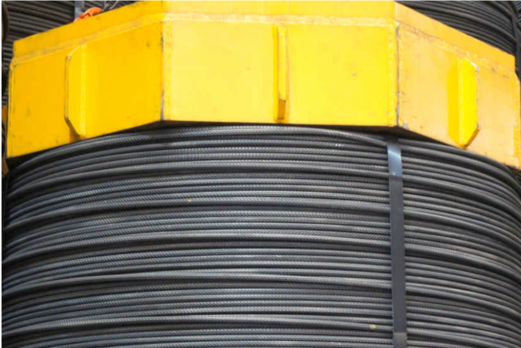
Figure 2: New rebar coil magnet on 5t load
