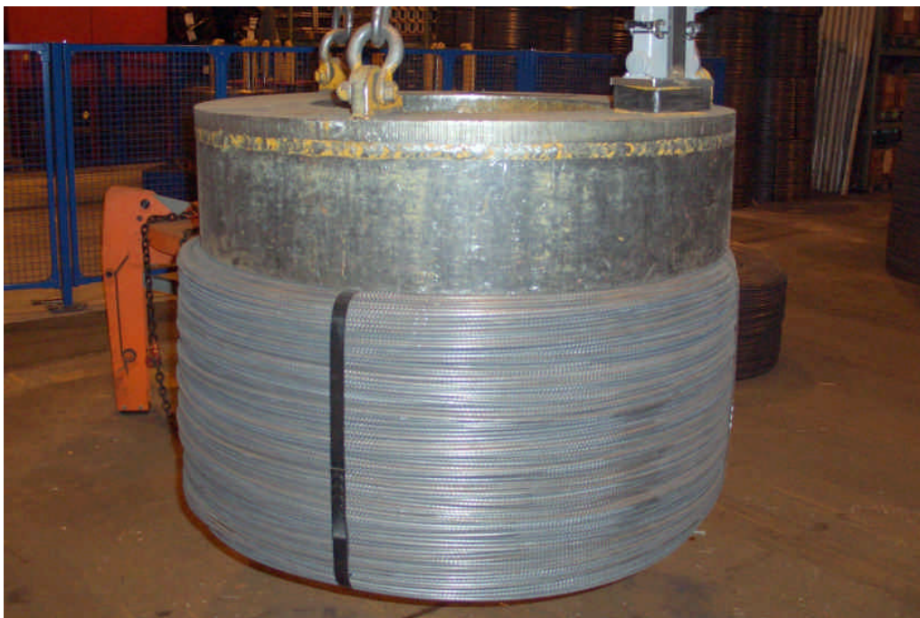
Figure 1: Magnetic lifting of a 3t, 1'200mm diameter rebar coil
