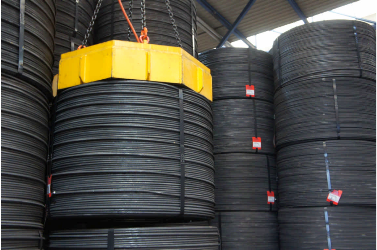
Figure 3: High storage density with magnetic stacking of rebar coils
