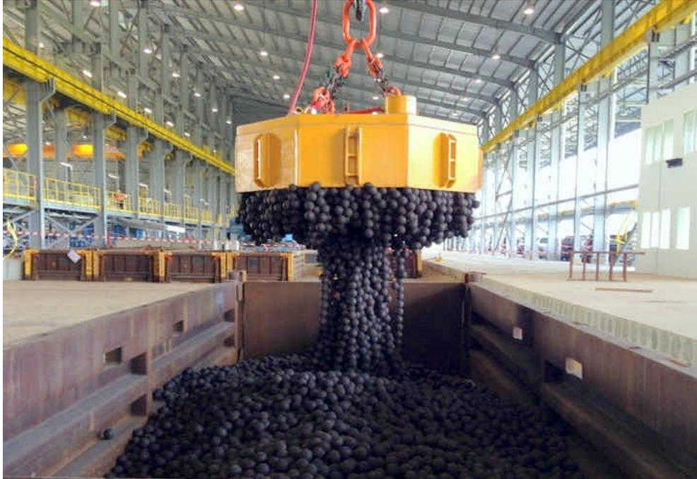
*Figure 3: Deep magnetic field even with low material density*
