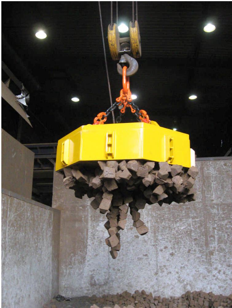
*Figure 1: Picking of a pre-determined weight of ingots*
