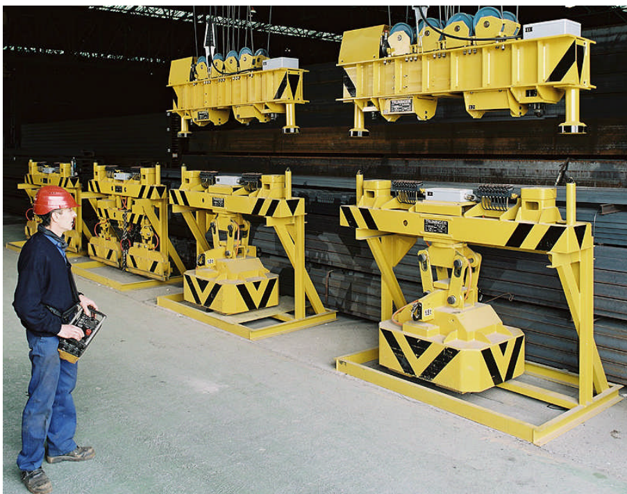
Figure 3: Quick coupling up of the section pack magnets for fast and efficient unloading of trains and ships
