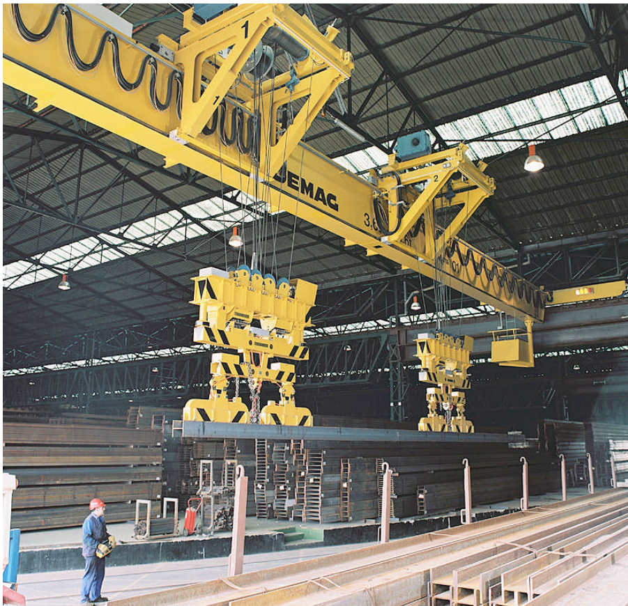
Figure 1: QuickChange™ system with lower spreader beams for handling individual sections in the prefabrication area
