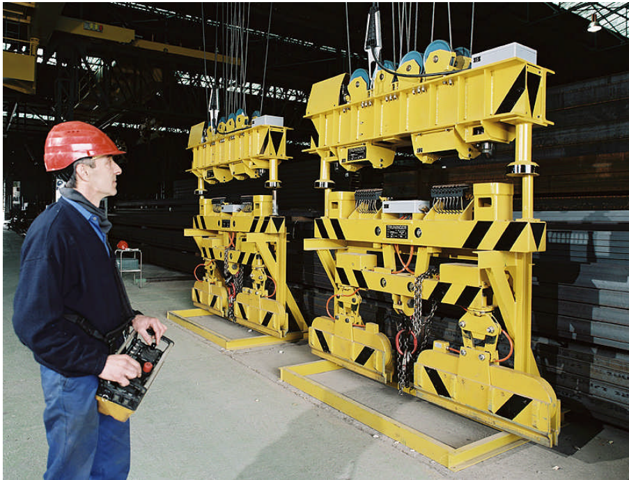
Figure 2: Automatic decoupling of the lower spreader beams for individual sections
