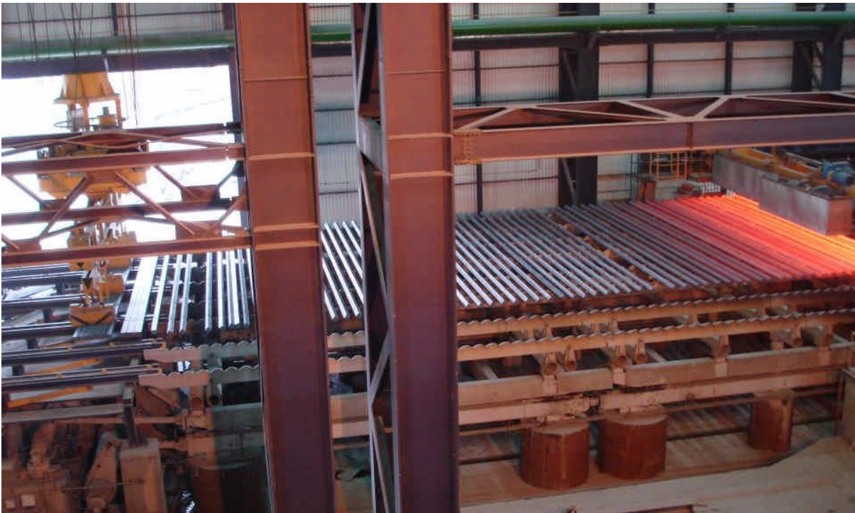
Figure 1: TRUNINGER-Magnet system for load temperatures up to 600°C
