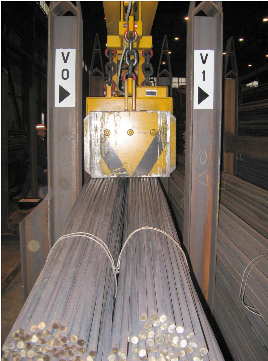
Figure 1: Storing bundles of still hot bars between uprights
