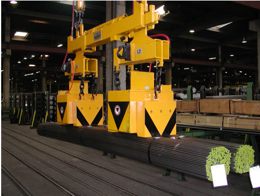
Figure 2: Magnet spreader beam for moving double bar bundles
