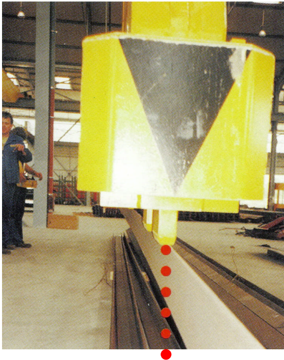
Figure 1: Extended anchor lifts a single section
