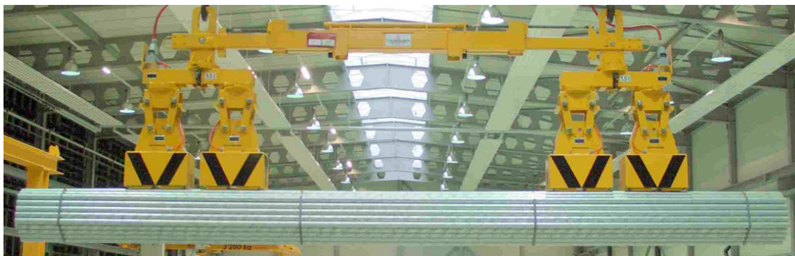
Figure 2: Magnets turned parallel to the load, lifting a bundle of pipes
