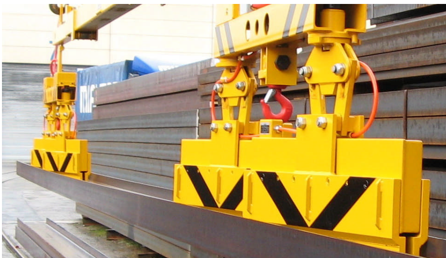
Figure 4: Slewing magnets set at a slight angle on a wide load
