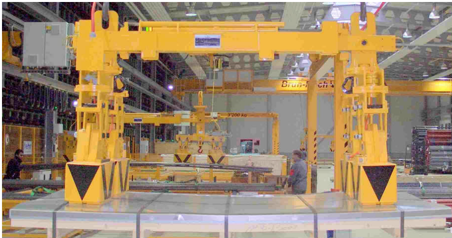
Figure 1: Magnets slewed by 90° on a pack of sheet metal
