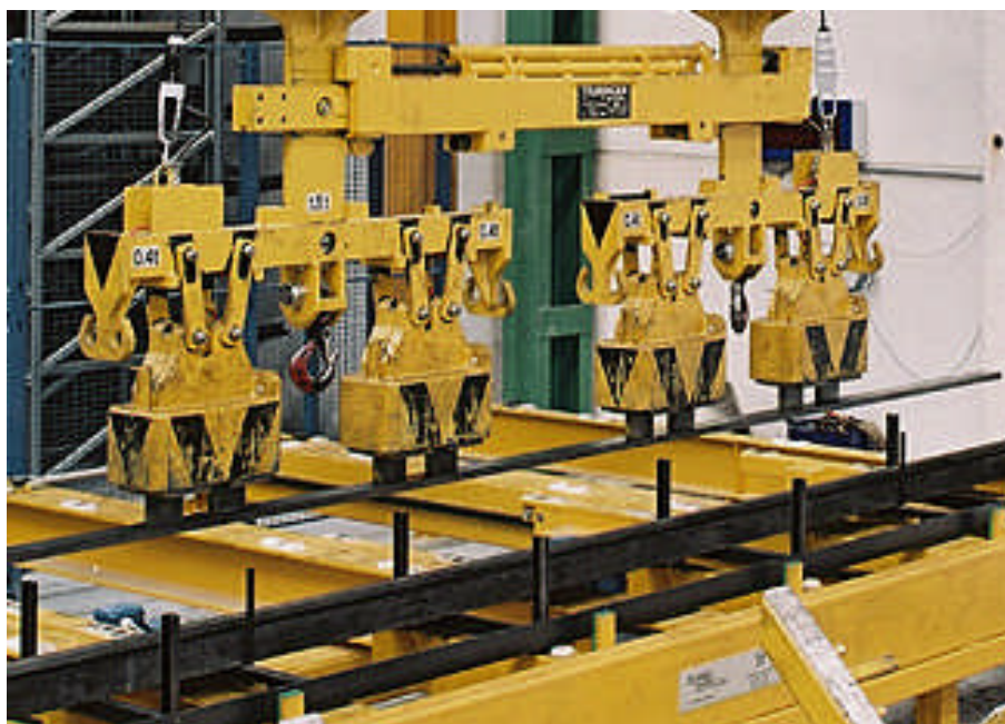
Figure 3: Picking a flat bar using the retractable anchors
