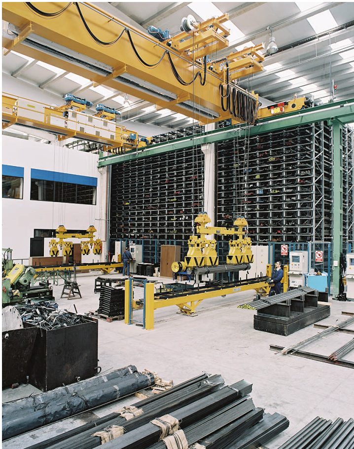
Figure 1: Putting bundles of bars into the storage rack
