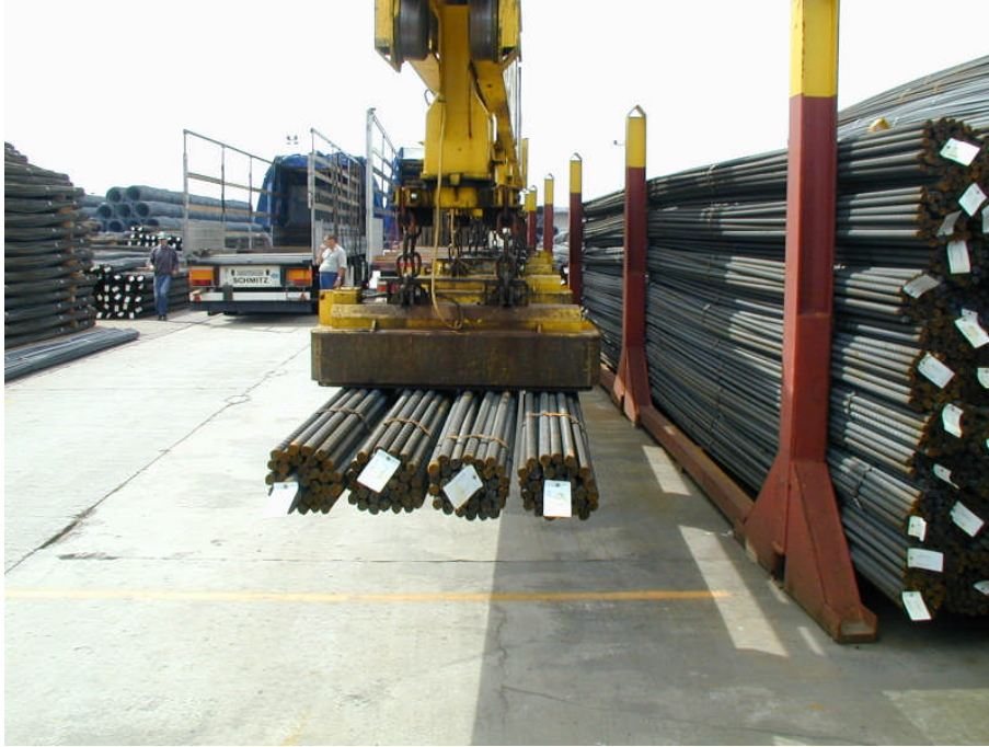
Figure 3: Efficient material handling with multiple-bundle transport
