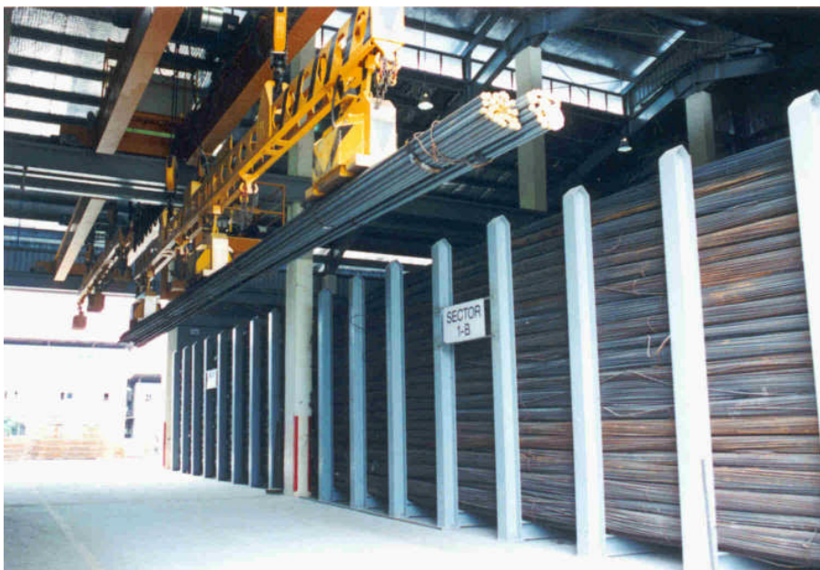
Figure 1: High storage density in a rebar warehouse
