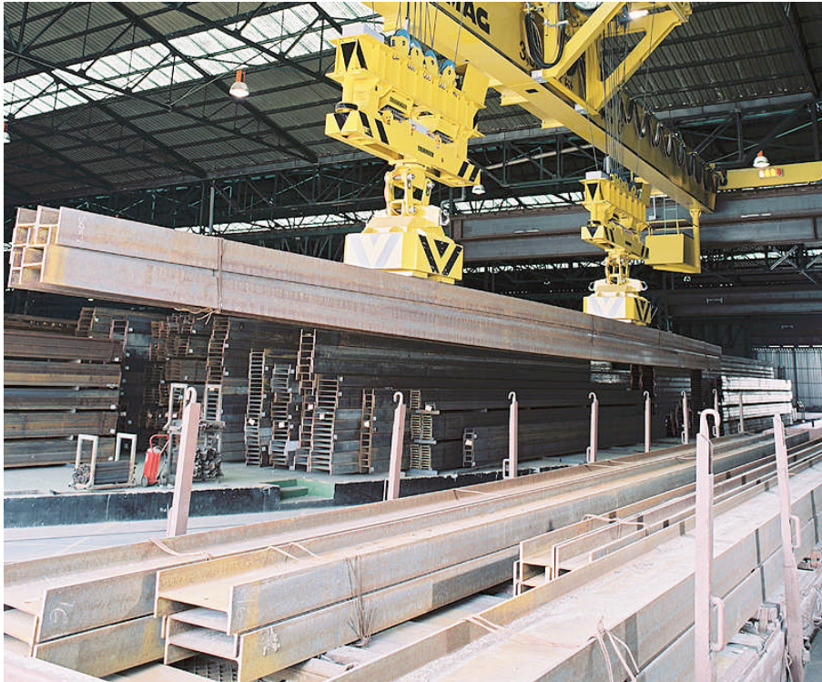
Figure 3: Two independent spreader beams with quick change systems unloading a railway wagon
