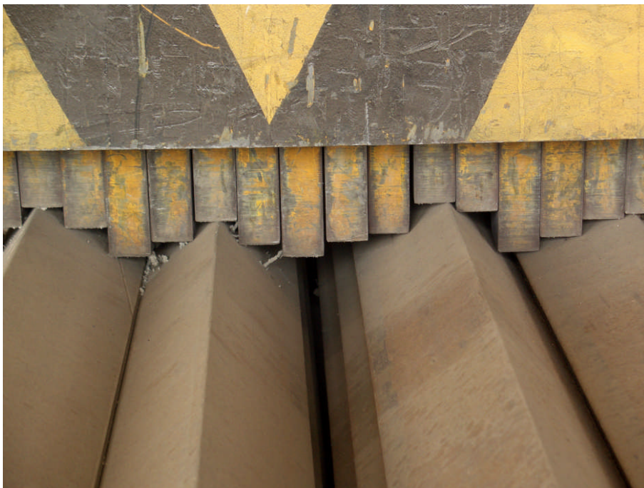
Figure 4: Finger poles adapt to the shape of a bundle of angled sections
