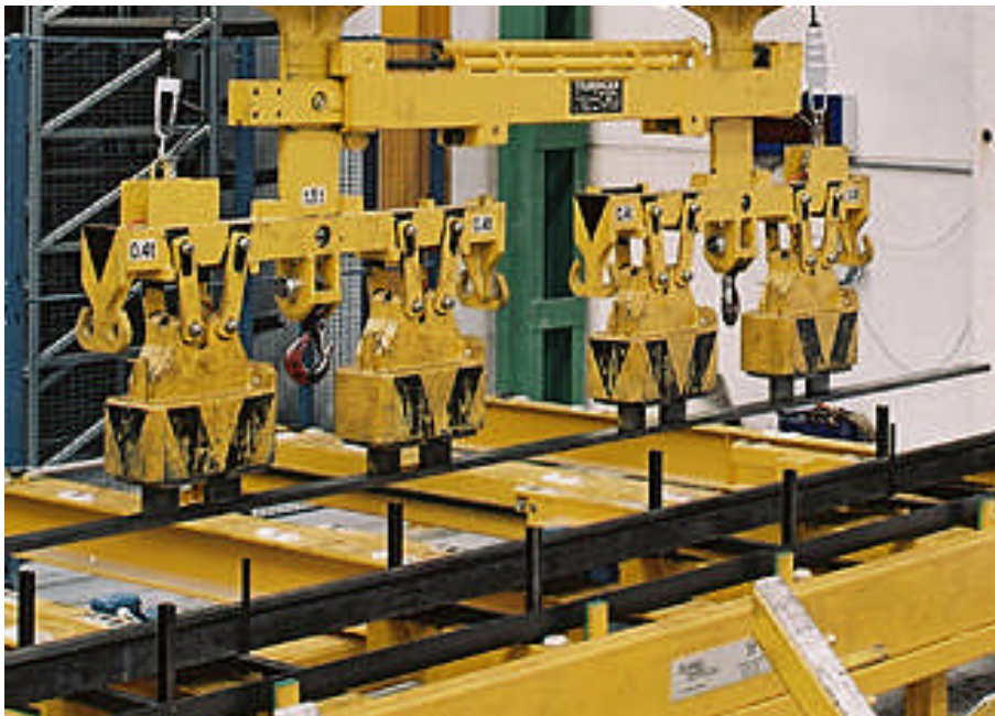
Figure 1: Swing-free order picking from a cassette
