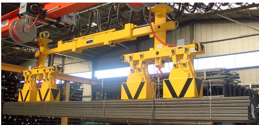
Figure 3: Passive telescope with two magnet groups lifting a bundle of hollow sections
