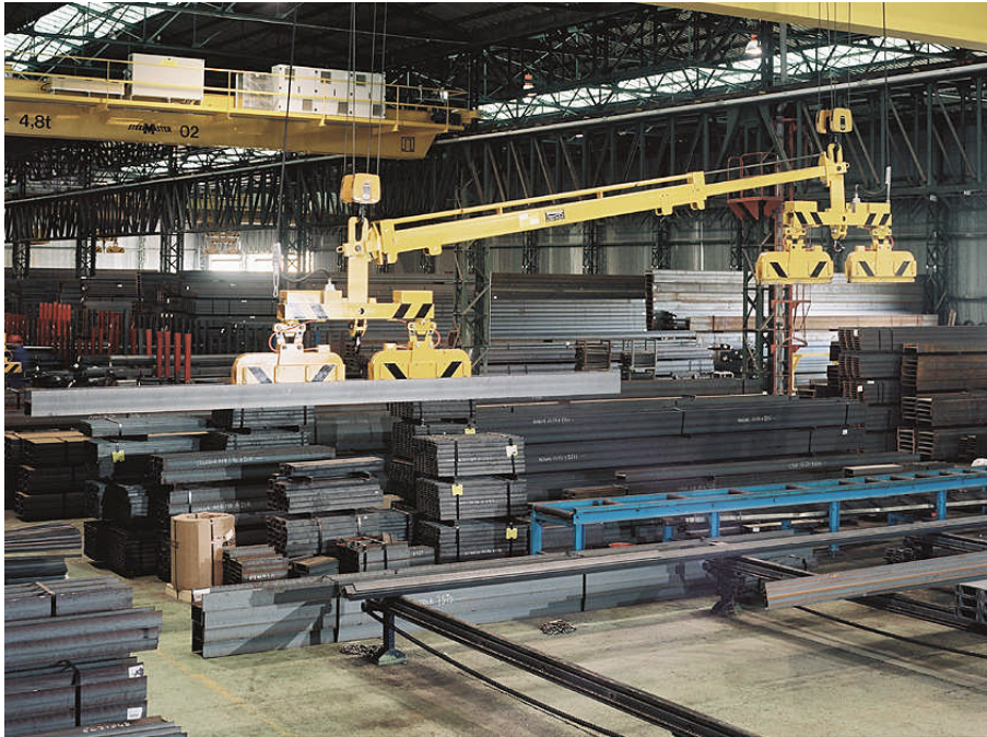
Figure 2: Lifting a short beam with a single magnet group
