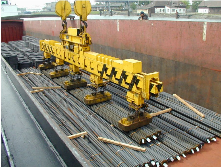
Figure 3: Active telescope unloading rebar bundles from a ship
