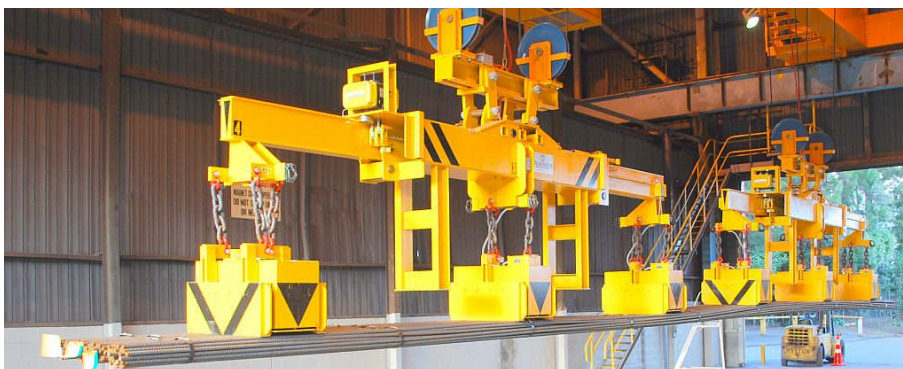
Figure 2: Two active telescopes transporting long rebar bundles
