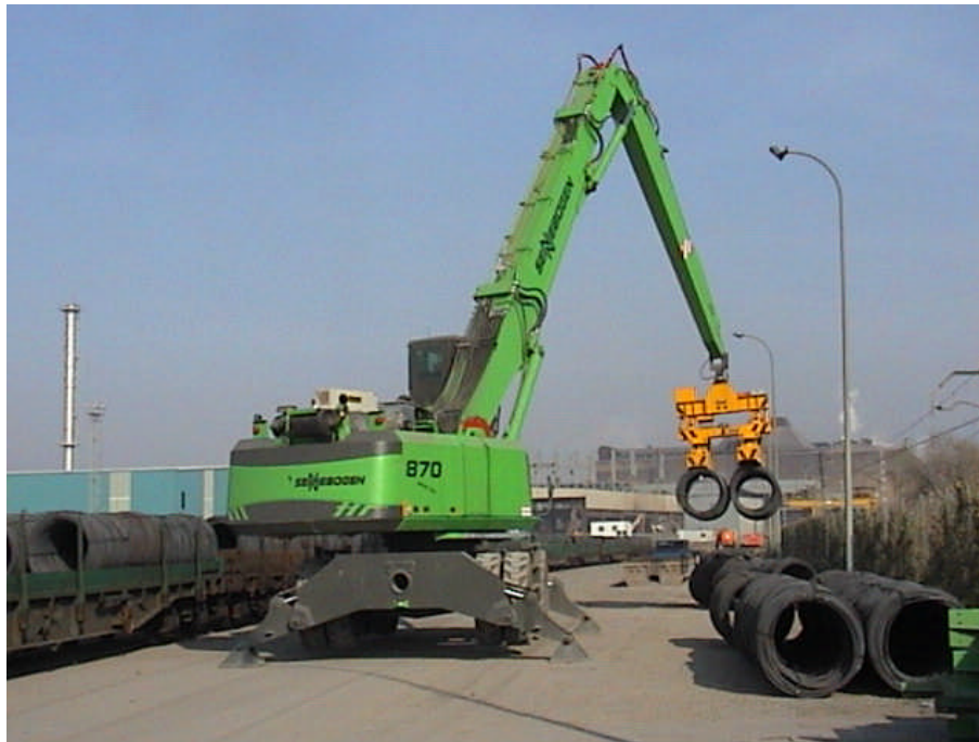
Figure 3: Mobile magnet system for lifting heavy rebar coils
