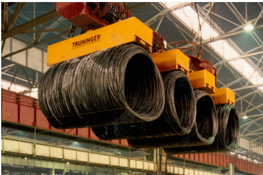
Figure 2: Magnetic transport of coils in a steel mill
