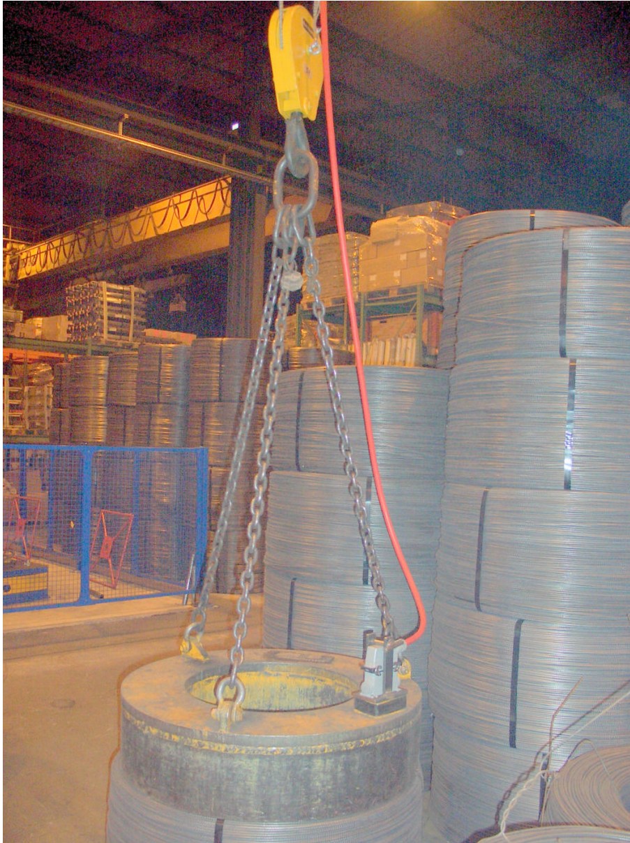
Figure 4: High-density storage achieved with a magnet system
