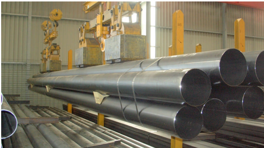
Figure 2: Lifting pipe bundles out of uprights using two individual spreader beams
