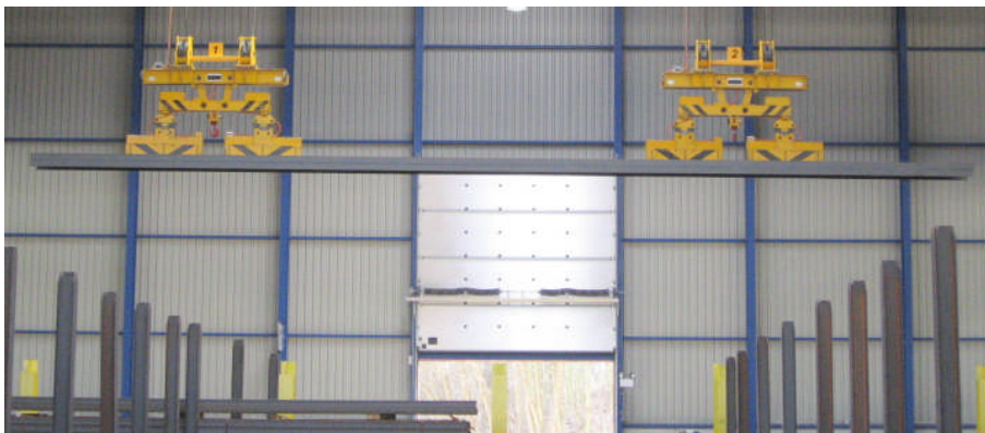
Figure 1: Two individual spreader beams carrying a long beam
