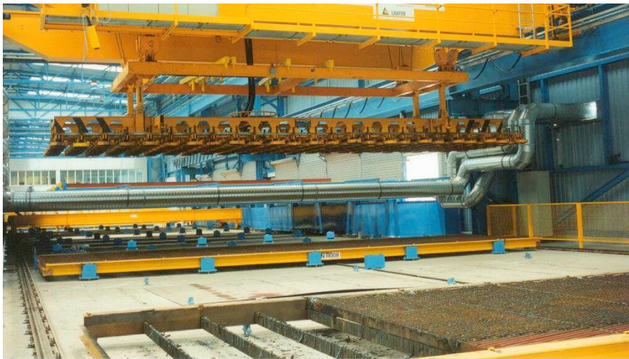
Figure 1: A “magnetic carpet” with 175 ring magnets for loading and unloading a cutting machine with plates of max. 12 x 3.5m
