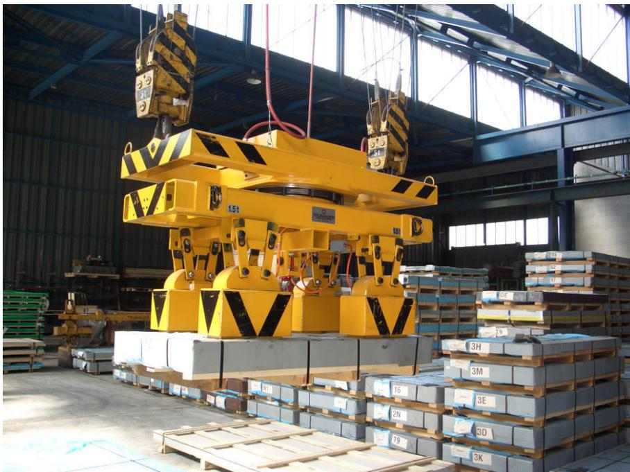
*Figure 1: Sheet pack on a spreader beam with travelling magnet groups and load slewing device*
