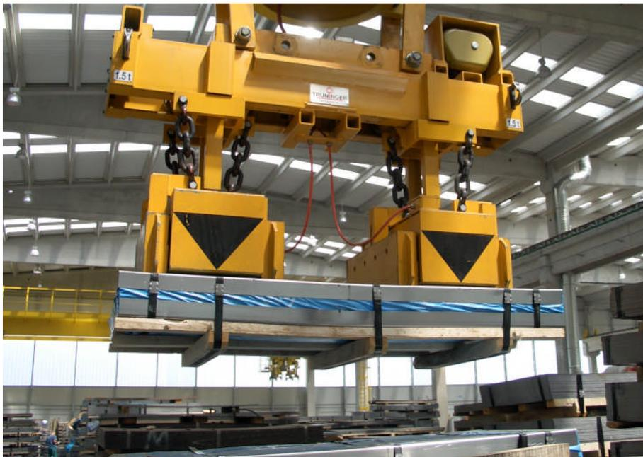
*Figure 2: Transporting a sheet pack using a deep-penetrating magnets*
