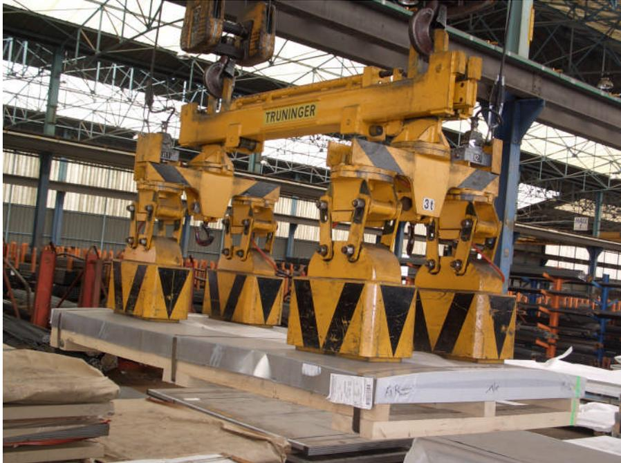
*Figure 3: Large sheets lifted using a passive telescope*
