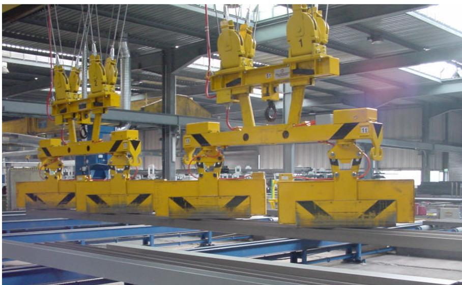
*Figure 3: Two individual spreader beams with anti-sway V-rope tensioning mechanism for lifting narrow beams*
