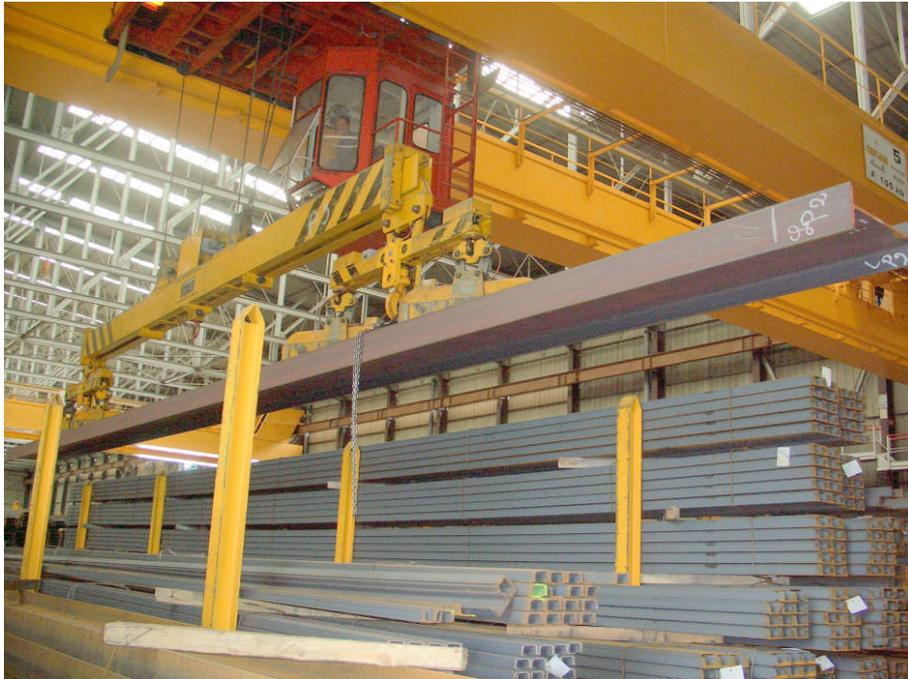
Figure 1: High-density storage using a TRUNINGER magnet system
