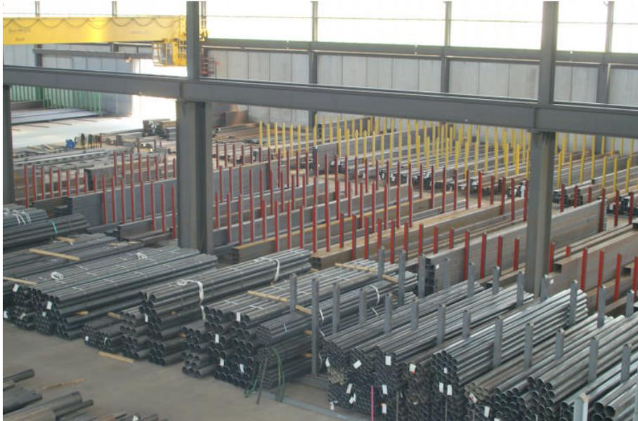
*Figure 4: Cost-efficient compact storage of long hollow sections using a magnet system*
