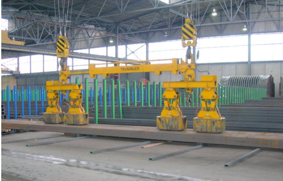
*Figure 2: Passive telescope used for transporting a layer of hollow sections*
