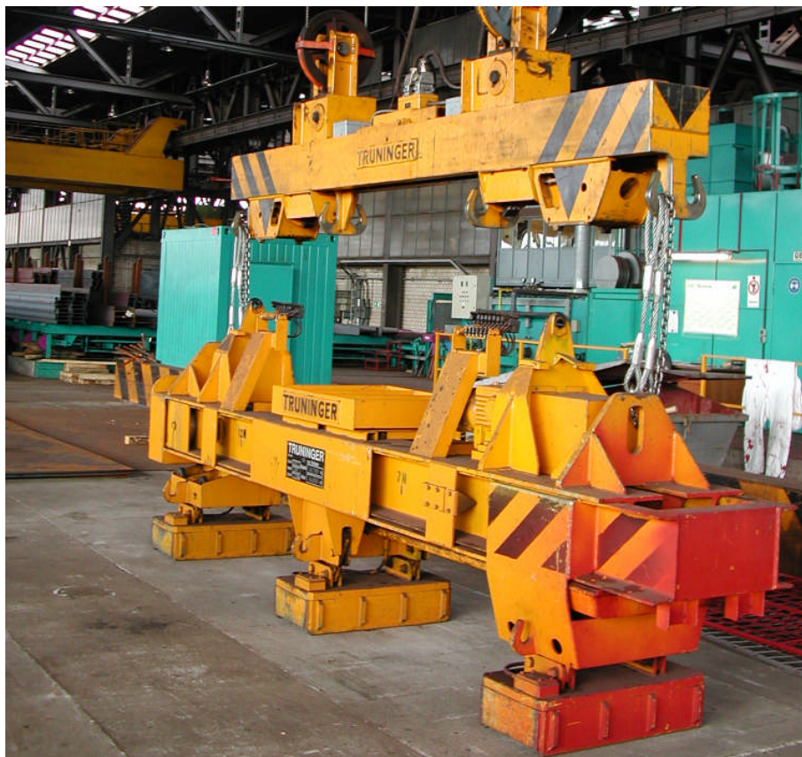
Figure 2: Active telescope with quick change device
