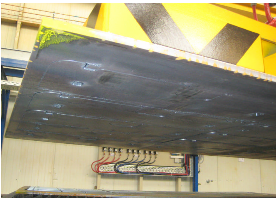
Figure 3: Off-cuts and scrap parts safely picked up in a single lift
