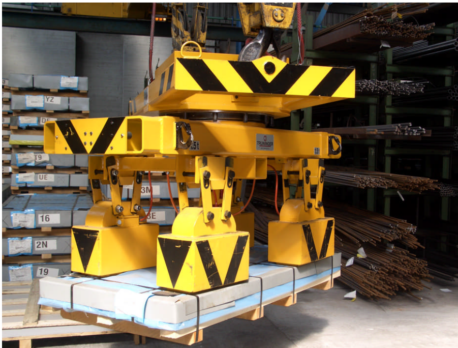
Figure 2: Magnet spreader beam with load slewing device
