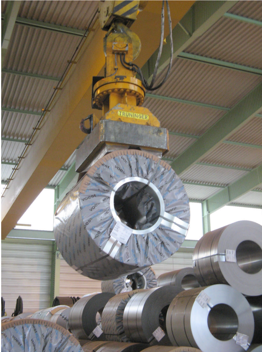
Figure 3: Load slewing device in combination with a coil magnet
