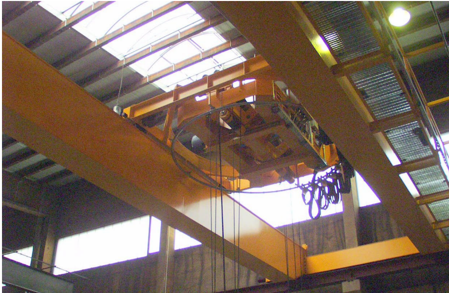
Figure 1: View of a slewing crab
