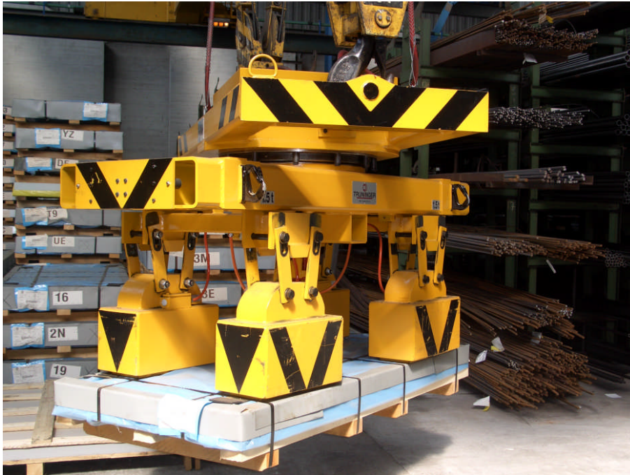
Figure 2: View of a magnet spreader beam with load slewing device
