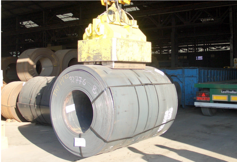
Figure 3: Moving a hot-rolled coil into store – Note the air gap
