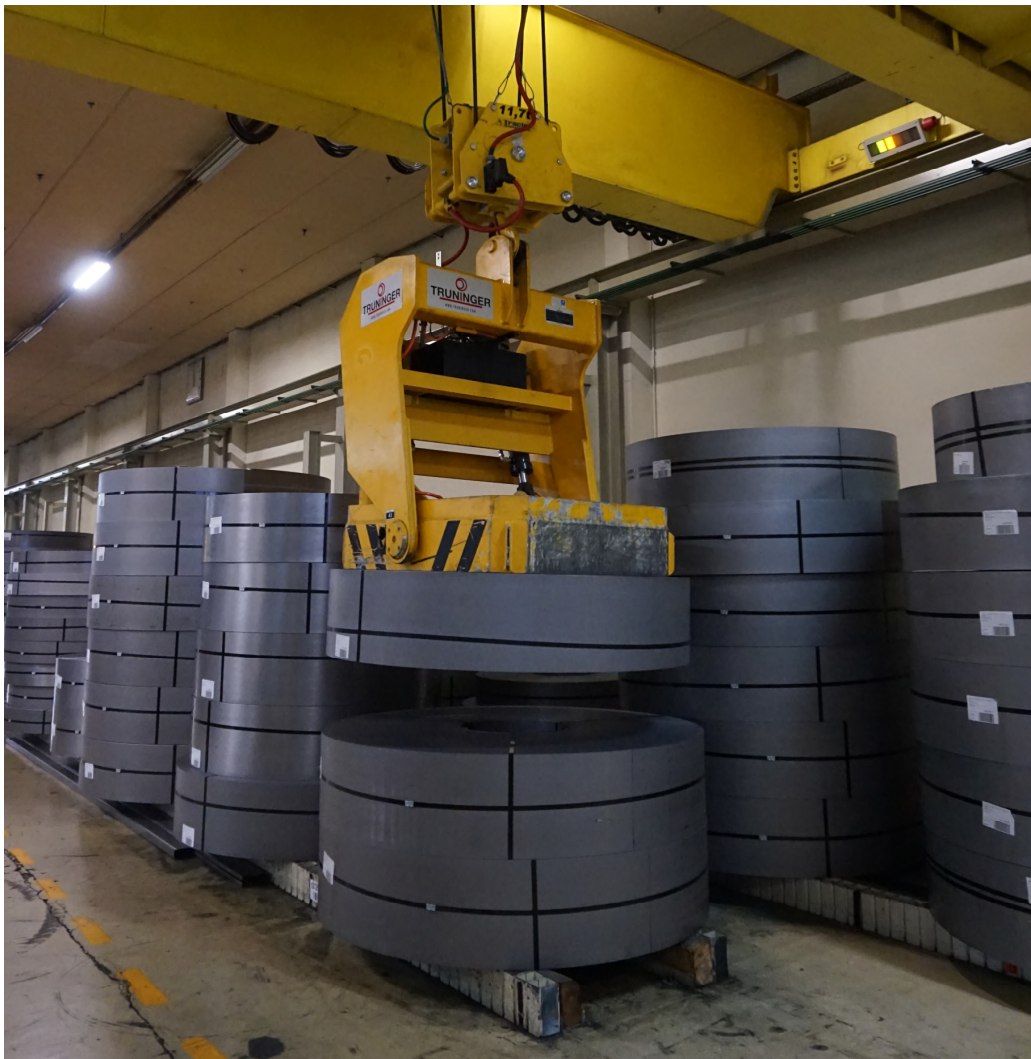
Figure 2: 8t Coil rotator in position – winding axis vertical
