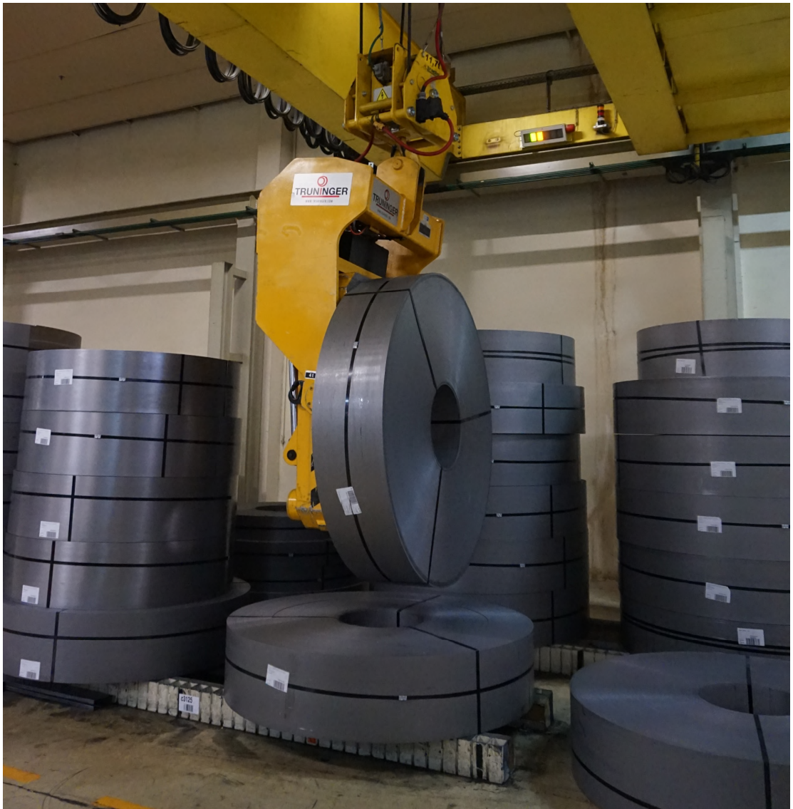
Figure 1: 8t Coil rotator in position – winding axis horizontal
