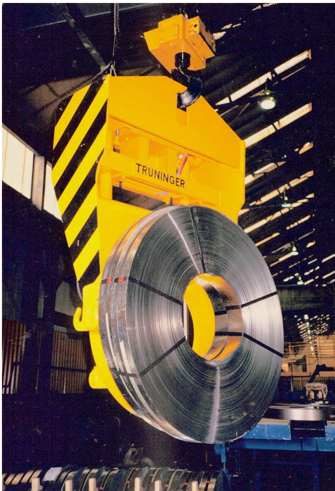
Figure 1: Coil rotator in position – winding axis horizontal
