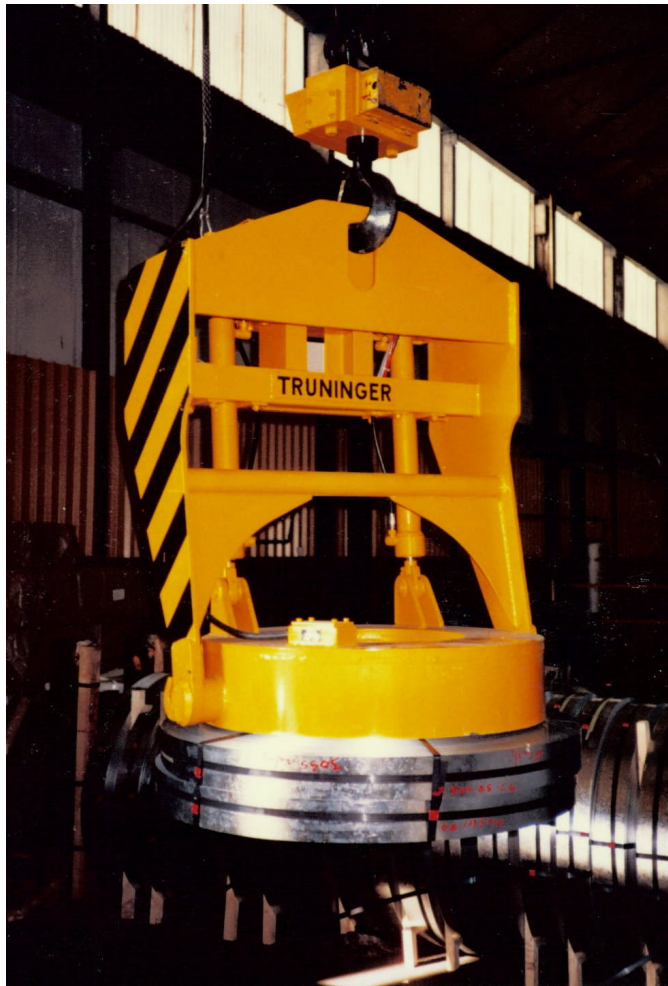
Figure 2: Coil rotator with ring magnet – winding axis vertical
