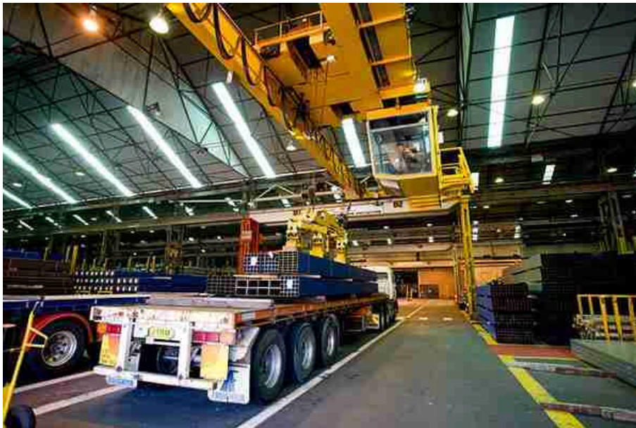
Figure 1: Carrying double bundles of thin-walled tubes for efficient loading of trucks at OneSteel in Australia
