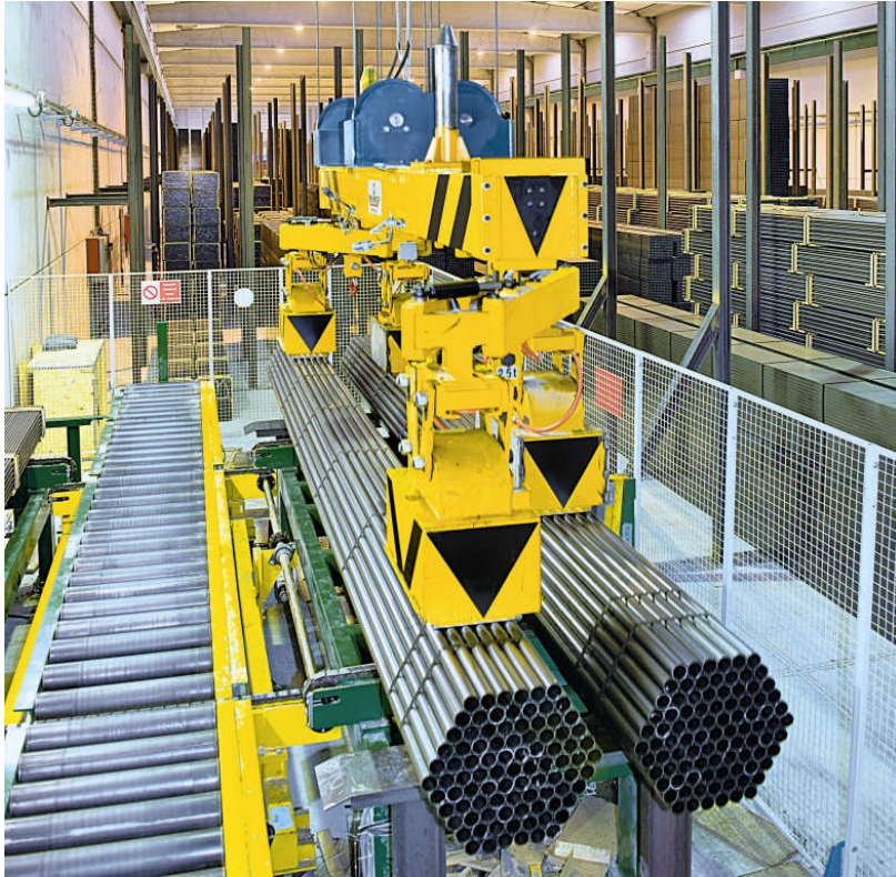
Figure 2: Clearing the end of a tube production line at Aratubo in Spain
