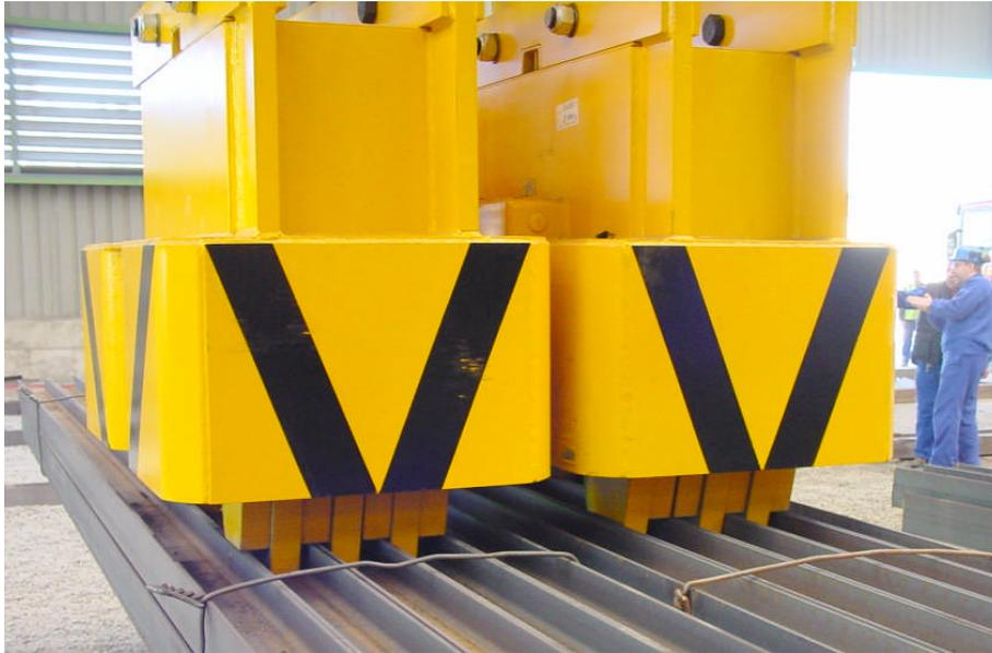
*Figure 4: Finger poles adapt automatically to the contours of the two H-profile bundles*
