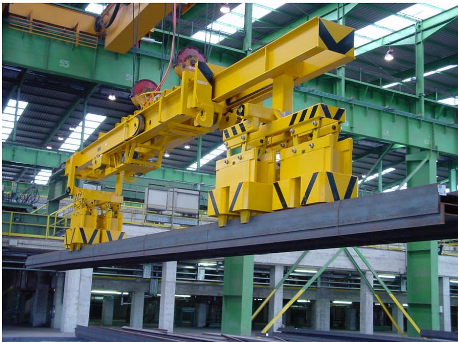
Figure 3: Dispatching and loading 3 bundles of beams in a single operation
