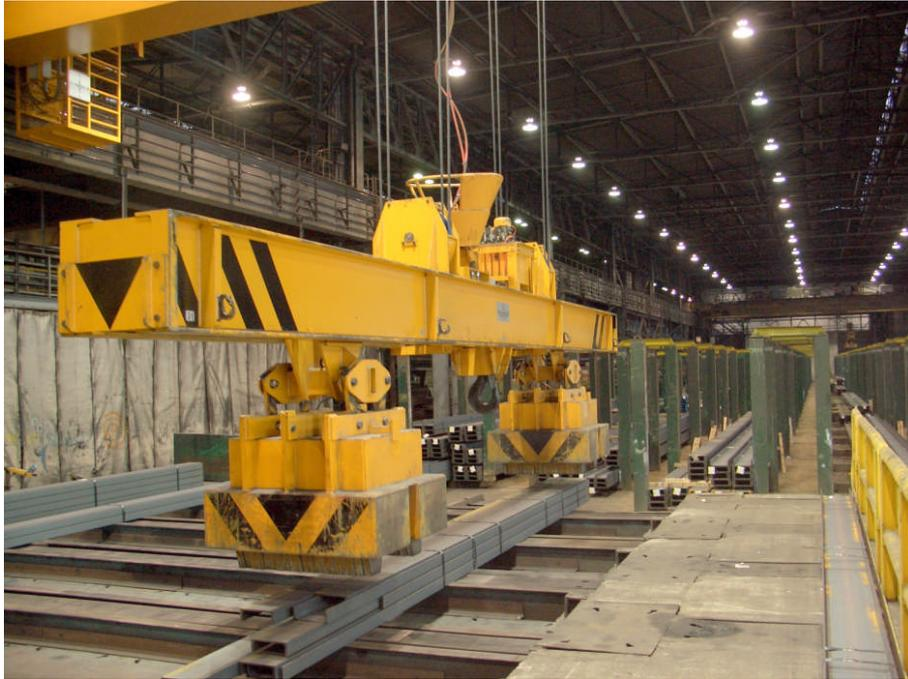
Figure 2: Magnet spreader beam used to move beam bundles to the dispatch storage area
