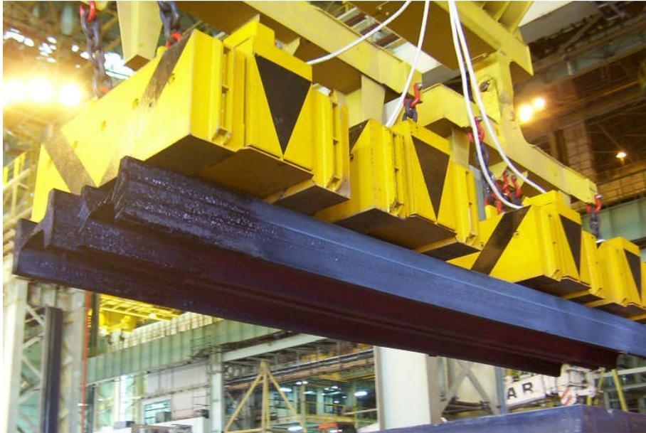
*Figure 1: Transporting layers of hot semi-finished beams*
