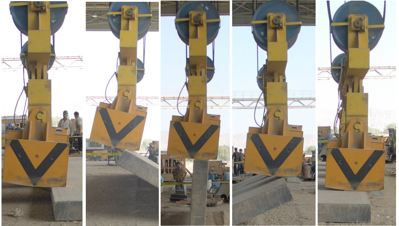
Figure 2: Turning a slab using magnets
