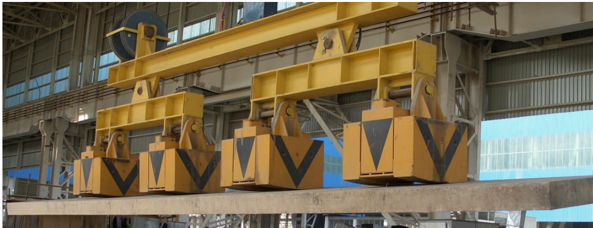
Figure 1: Slab-turning magnets taking a slab from a stack for further processing
