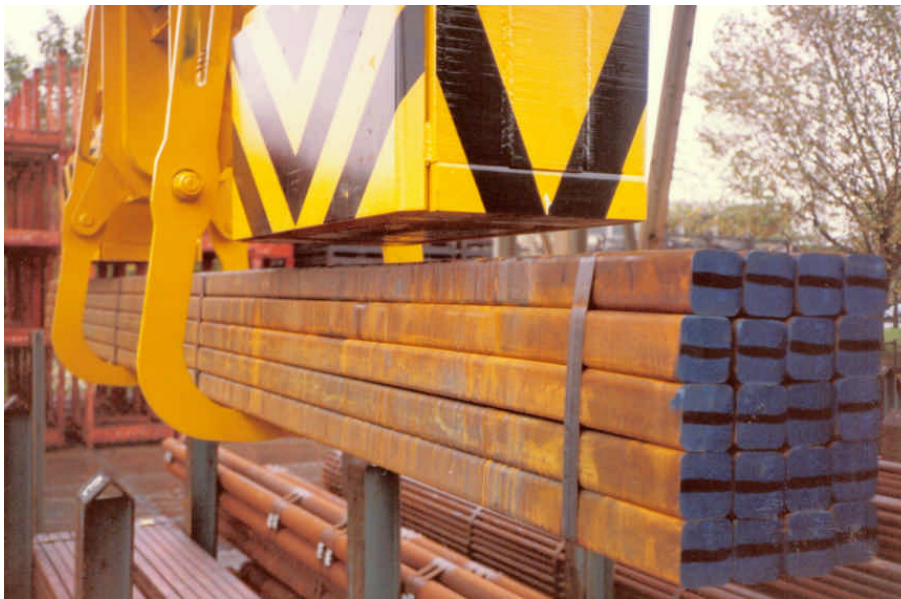
Figure 1: Safety gripper with secured load
