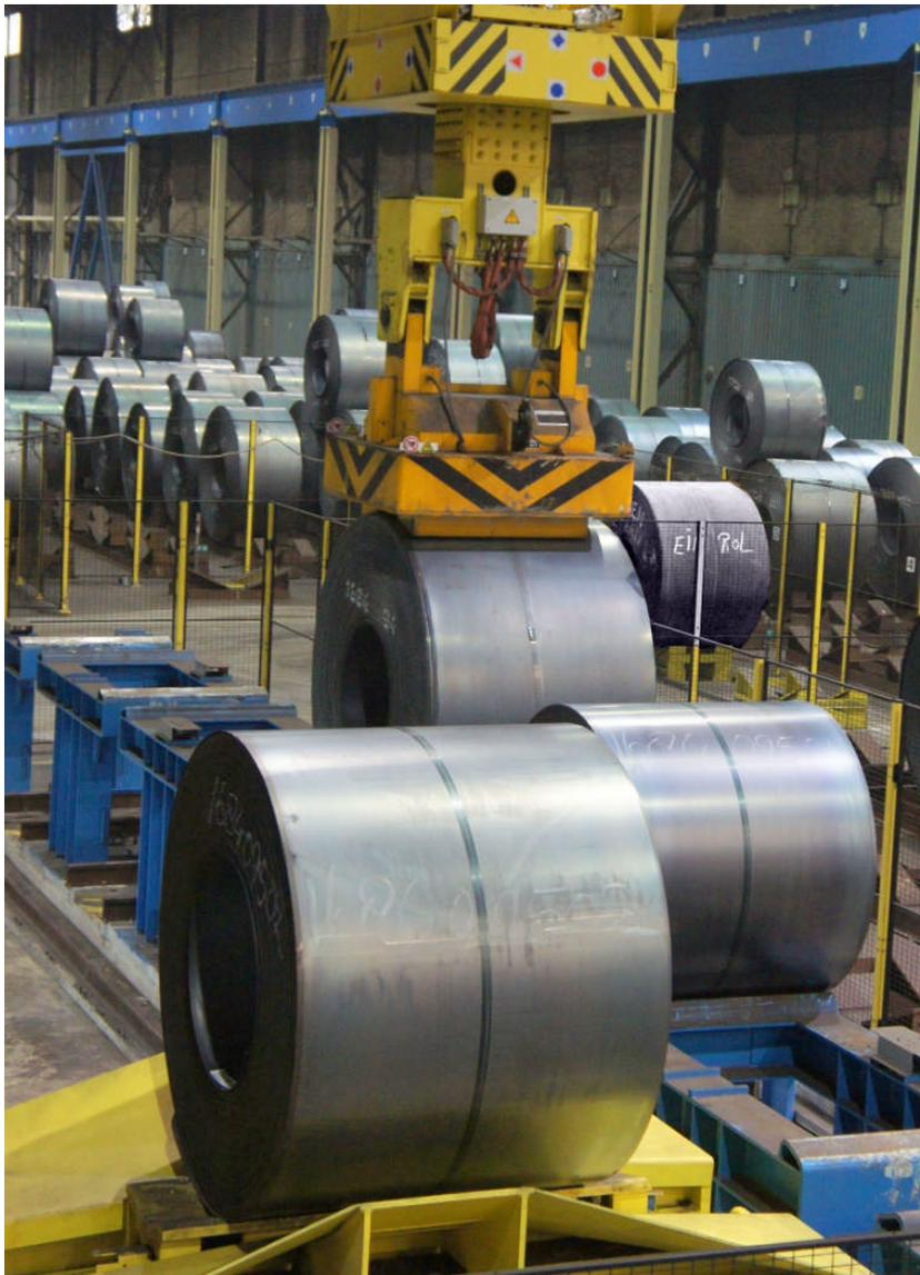
Figure 4: Coil being prepared for placement on the transfer carriage
