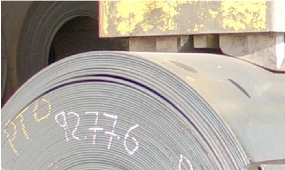
Figure 1: Air gaps in windings of hot-rolled coils
