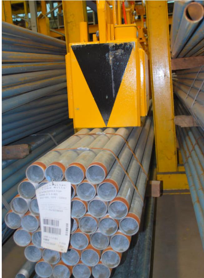
*Figure 2: Effortless handling of tubes in narrow storage compartments thanks to minimal side attraction*
