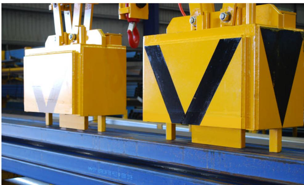
*Figure 3: Precise picking of individual tubes thanks to the ingeniously simple retractable pole anchor concept from TRUNINGER*
