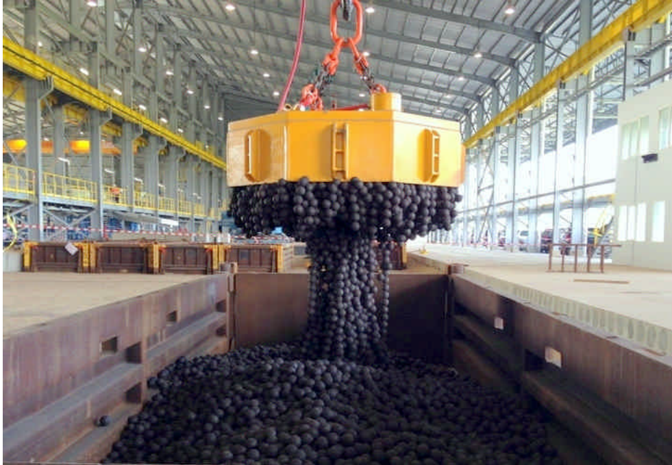
Figure 3: Deep magnetic field even with low material density
