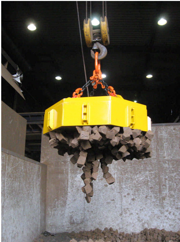
Figure 1: Picking of a pre-determined weight of ingots
