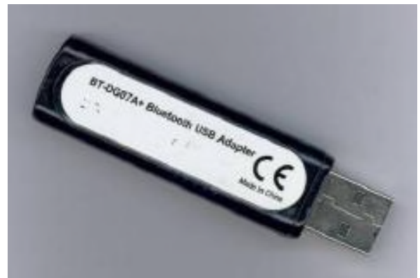
external Bluetooth adapter Truninger part no. E12230
